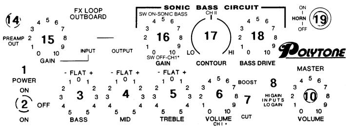
CH II SONIC BASS CIRCUIT - three pots control the Sonic Bass circuit and work in conjunction with each other: GAIN - CONTOUR - BASS DRIVE
